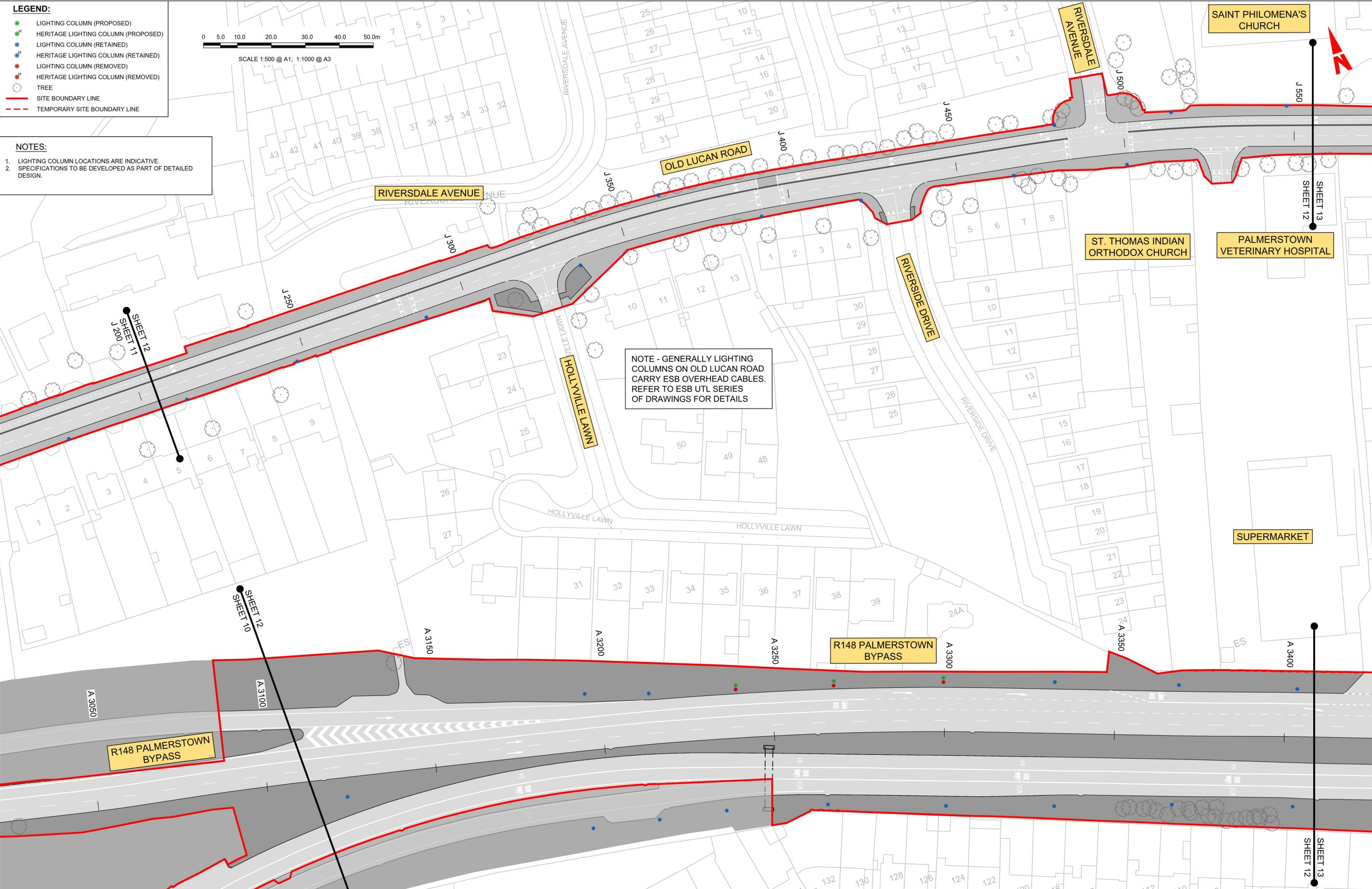
NOTE - GENERALLY LIGHTING COLUMNS ON OLD LUCAN ROAD CARRY ESB OVERHEAD CABLES. REFER TO ESB UTL SERIES OF DRAWINGS FOR DETAILS
